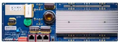
RS485 Communication between battery and server Baud rate:9600bps RS485 interface Communication between parallel packs or EMS and PC Baud rate:9600bps
